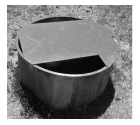
Figure 30 – Float Tank with Lid
