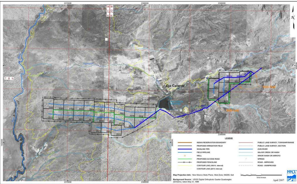
PIA Map 2: Field and Irrigation System Layout for Plumasano Irrigation Project
